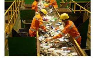
Workers sorting out recyclables at the manual sorting line at SembWaste's Materials Recovery Facility
