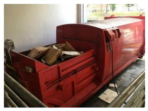
Packaging material is segregated for recycling. Image shows cardboard compactor where cardboard boxes are placed and compressed for recycling.
